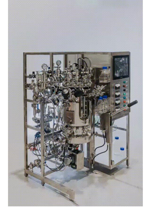
Ensuring top-notch maintenance for our stainless steel bioreactors, we've introduced an adjustable and pivotable lid lifting device. This design facilitates effortless access to the bioreactor, whether for cleaning or upkeep. The lid's pivoting motion guarantees easy reach to all ports on the top lid, and safe, unobstructed entry to the vessel itself.
