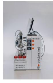
clean magnetic mixers and advanced peltier systems. Each reactor operates independently, allowing for two separate fermentations. The standalone design requires only electricity, making it ideal for researching the best fermentation process parameters. Plus, its condensers come with Peltier elements for exceptional exhaust gas cooling without the need for circulating water. Read More
