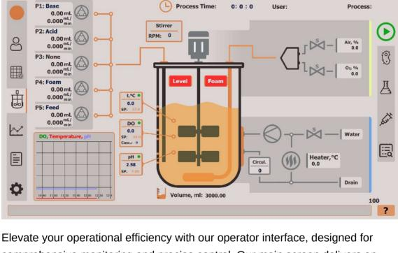
comprehensive monitoring and precise control. Our main screen delivers an intuitive platform to monitor key process parameters, including setpoints, sensors, valve status, and alarms. Dive deeper with the settings screen, allowing tailored parameter configurations and advanced PID controls covering essential processes like heating, DO enrichment, and cooling. Experience streamlined process management, optimal performance, and a user-centric environment with our state-of-the-art solution.
